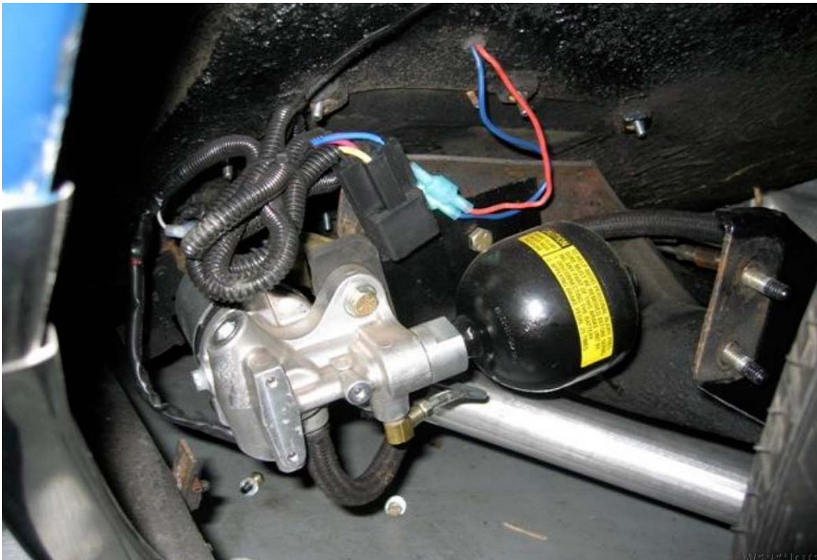
Electric Brake Booster, installed on HK1CD5 in same location as original Vacuum Booster (It is normally hidden by the original stone shield, which was removed to show mounting detail.)
