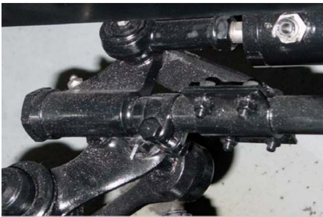
Center rod support brace, attached with 4 bolts
