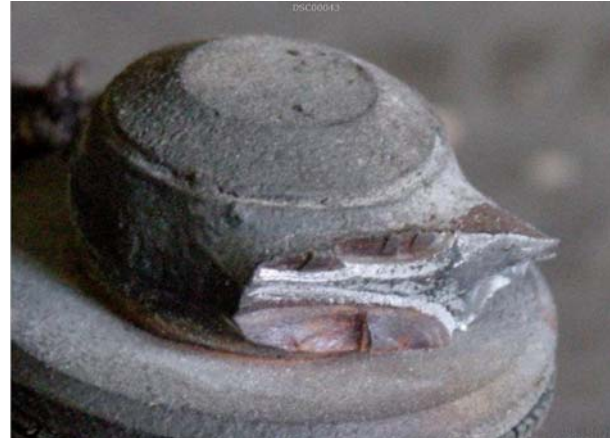
Close-up of FV4 Pitman arm break near joint
