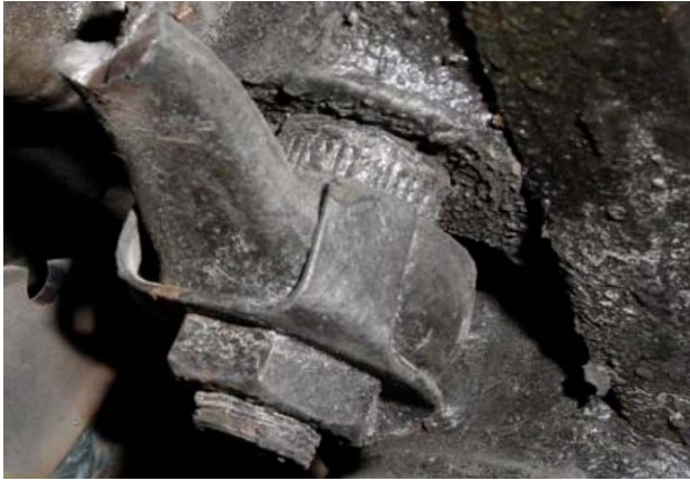
FV4 Pitman arm, broken while driving
